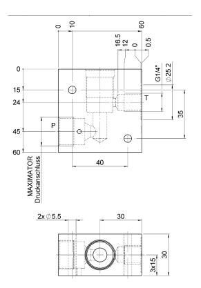
Dimensional drawing with pressure relief cartridge (Cartridge not included in scope of supply)
