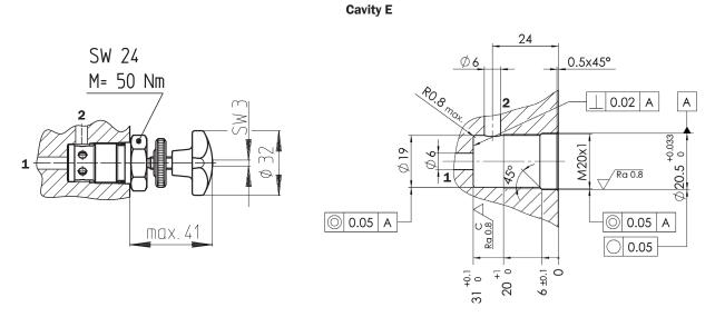
Cartridge check valve see technical data sheet ZP700/BL700/RV700
