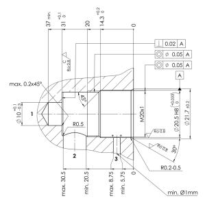
Steel yield strength Rp0.2  $\geq$  450 N/mm<sup>2</sup> elongation at fracture As  $\geq$  10% \* Flat chamfer or rounding max. 0.5 wide
